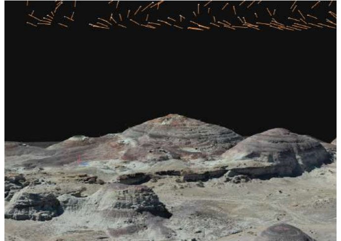
Figure A.12: Point cloud reconstructed by RealityCapture. The position and direction of the aerial images are visible in orange. The region scanned is the Marble Ritual region (38.4036° N, 110.7883° W).
