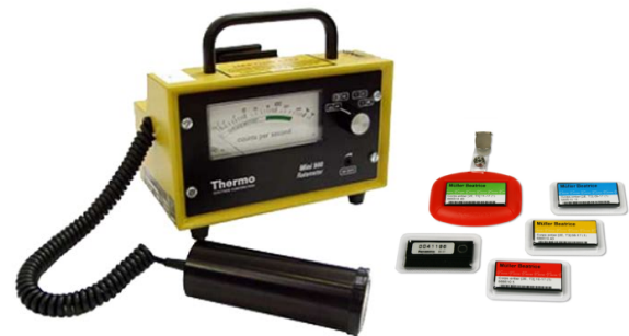
Figure 1 – NaI scintillator (left) and personal passive dosimeter (right) [3].
